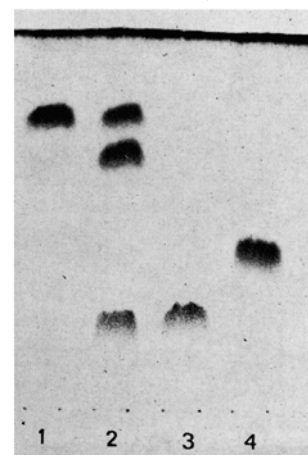
Fig. 3. TLC of diglyceride acetates on a "silver plate." Solvent: benzene-chloroform (9:1). 1: 1,3-Dipalmitin acetate. 2: Acetolysis product of a mixture of 1,3-dipalmitin and 1,3-diolein (the second spot is 1,2-dipalmitin acetate). 3: 1,3-diolein acetate. 4: A monoenoic 1,2-diglyceride acetate.
